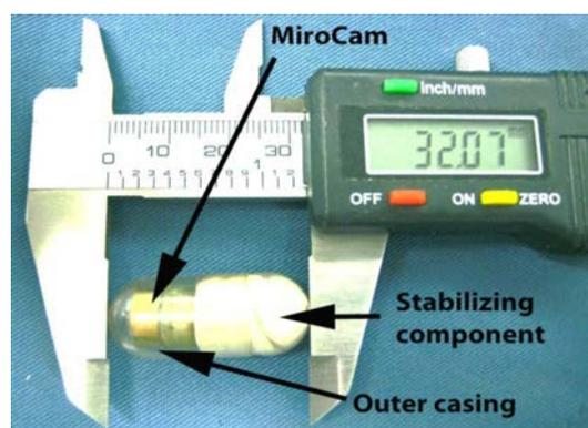
Fig. 2. Assembled self-stabilizing capsule endoscope. Length (in millimeters) is measured by a caliper.
