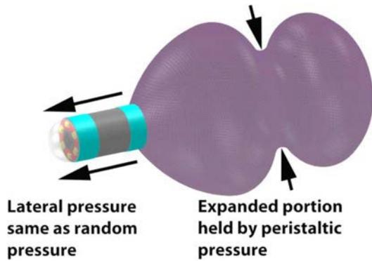
Fig. 3. Worst-case scenario for the stabilizing component where one end is held and the other is pulled by lateral and circumferential forces.
