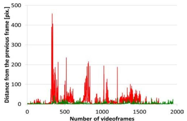
Fig. 10. Distances between the locales in successive video frames for the unstabilized (red) and the stabilized (green) capsules.
