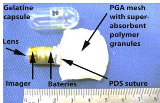
Fig. 1. Steps in assembling the self-stabilizing capsules. The expandable component made from permeable PGA mesh filled with superabsorbent polymer granules was attached to a reduced version of the MiroCam capsule containing only the batteries, the imager, and the lens. Subsequently, the entire implement was put in a gelatin capsule.
