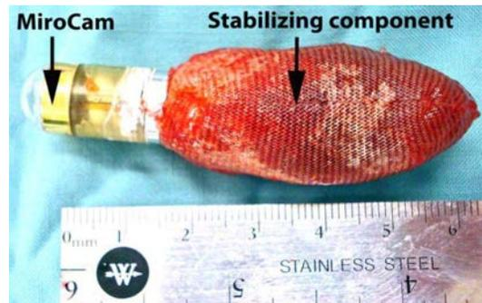
Fig. 6. Fully expanded self-stabilizing capsule endoscope. Due to its permeability, the mushroom-like tail swelled immediately after the degradation of the gelatin cover to provide stabilization to the imaging module.
