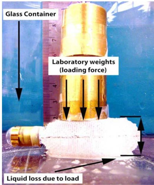
Fig. 4. Experimental setup for measuring maximum swelling pressure. From a certain laboratory weight on, the expanded stabilizing component started to decrease its volume. The contact surface area between the laboratory weight load and the expandable component was kept constant at 1 in<sup>2</sup>.
