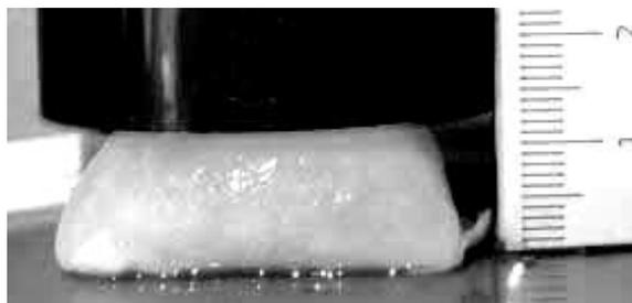
**Figure 2.** After expanding, Zalak<sup>®</sup> did not reduce its dimensions to less than 1.5 cm in any direction under force of 1.5 N (shown as a weight load on top) regardless of the pH dynamics of the simulated gastric medium.
